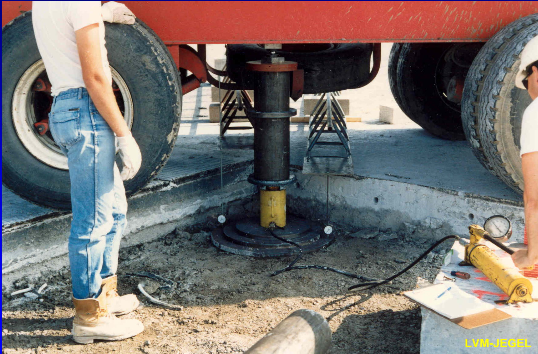
TYPICAL PLATE LOAD TEST ON RUNWAY
